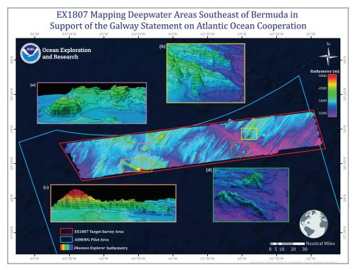
Kongsberg EM302 bathymetry data collected on NOAA Ship *Okeanos Explorer* during EX1807. During this expedition, the *Okeanos Explorer* mapped a focused survey area over 20,500 square kilometers, an area larger than Massachusetts. Exploration mapping revealed a complex seafloor structure, including distinct conical features, a true seamount, and southwest/northeast trending linear ridges. *Image courtesy of the NOAA Office of Ocean Exploration and Research*.
